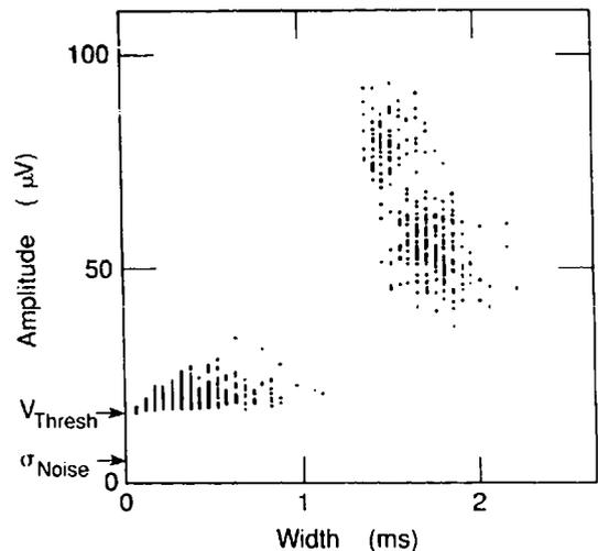
Fig. 7. A scatter plot of amplitude vs width for signals from tiger salamander retinal tissue recorded on a single electrode. The threshold voltage and  $\sigma_{\text{noise}}$  are also shown.
