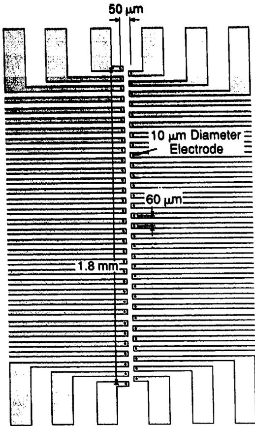
Fig. 5. The layout of the 61 electrodes for a quasi-one-dimensional retinal readout array.
