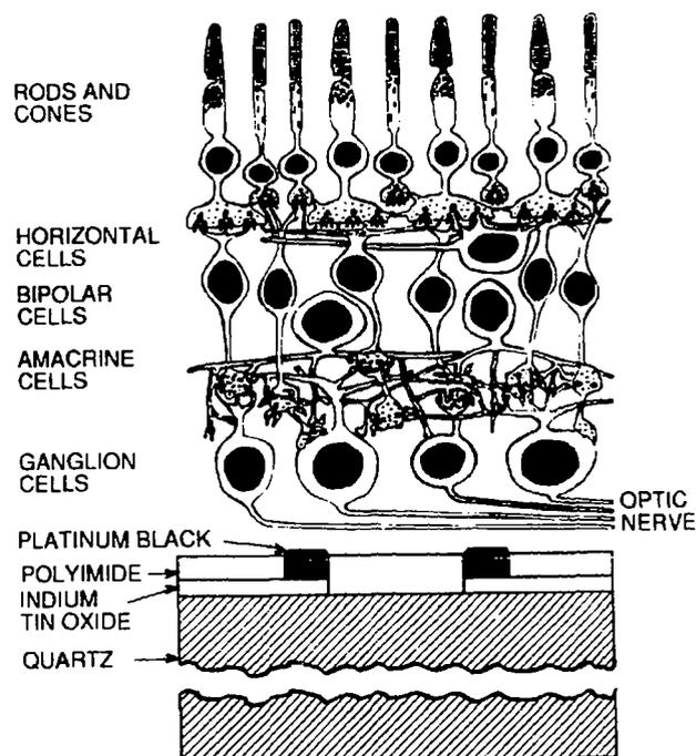
Fig. 1. A schematic view of the retina placed on top of an electrode array. The vertical dimensions of the electrode array as drawn are not to scale; the correct dimensions are given in the text.
