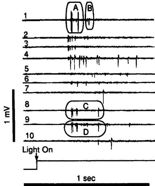
Fig. 6. The signals from tiger salamander retinal tissue recorded on 10 separate electrodes. The onset of a 2-s long light signal is indicated.
